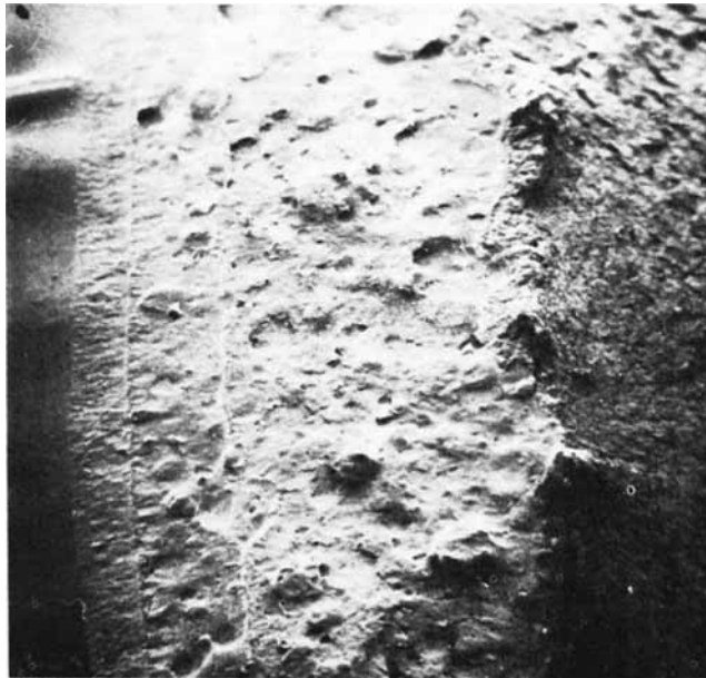
Fig. 7. PVC fracture surface, notch, low blow, and fast crack, \times 25 .
